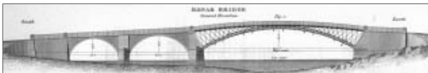
Bonar Bridge – elevation (Telford) [27]
