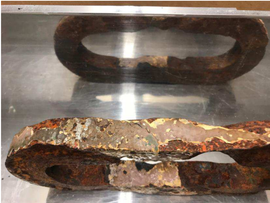
Microwave Spectroscopy Testing at Adrok's laboratory of an 1820 UCB iron coupling positioned in centre of the ADR 16 Channel Polarisation Test Chamber ©Adrok
