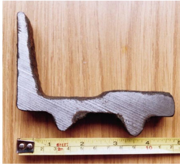
Fig. 5. Worn rail section at mid-length (far left) and replica plate-way detail (left) (now in the ICE museum at Heriot-Watt University)
