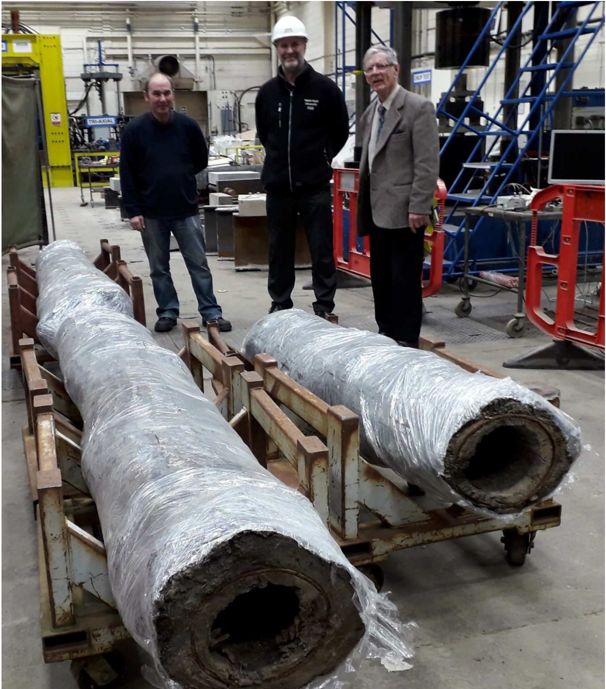
Wooden pipes from George Square drying out in EGIS Workshop at Heriot Watt University. [L to R] Tom Stenhouse Technician , Tom Ferguson Technical Services Manager & Roland Paxton ©S.Purves
