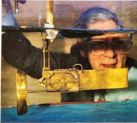
[61] David's Adie & Son tachometer being used by the author to measure underwater current velocity at Heriot-Watt University, to be read off.
