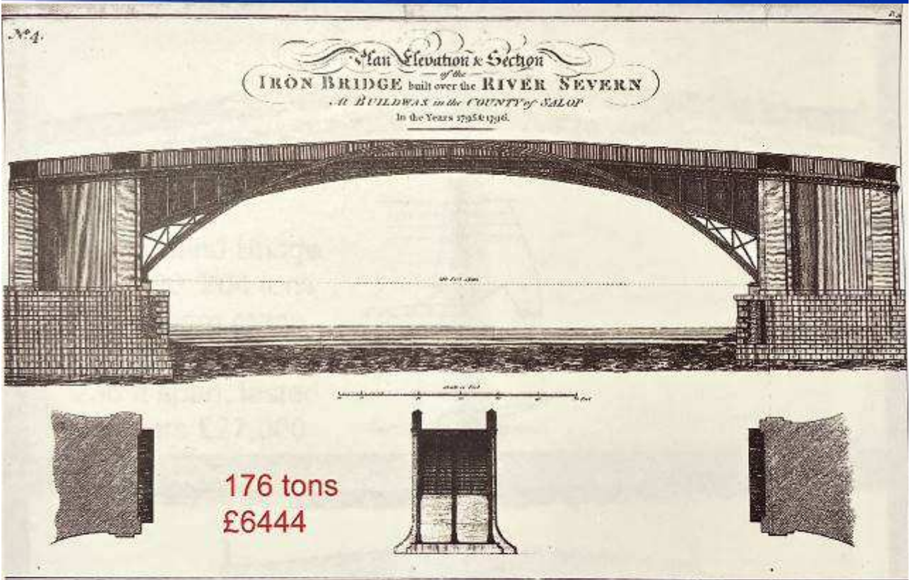
Buildwas Bridge, Salop, Telford 1796, had a 30% greater span than the Iron Bridge for half its weight
