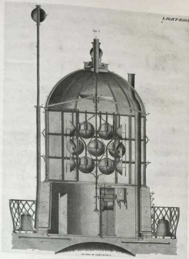
Light-room, with revolving array of silvered copper reflector lamps, signal ball, fog bells and ornamental iron balcony railing. (3, pl. XX)
