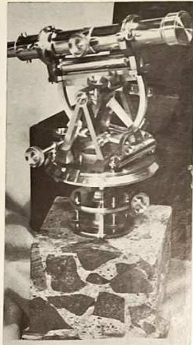
Figure 4. Specimen of early cement grouted macadam concrete—1878. The concrete was formed on a blinded and rolled stone bottoming 6 in thick as follows: A 4½ in thick layer of 1½ in whin road metal was spread uniformly over the bottoming and grouted with a mixture of fine gravel riddled out of Fisherrow gravel and Robin & Co's best (Portland cement). The cement used was to be capable of sustaining a tensile strain of 600 lb on the superficial area of 2½ in of the standard test block after being immersed 7 days in water. The grout was mixed in a patent steam mixing machine and then spread, beaten and "equalised" into the road surface" in a most careful and tradesmanlike manner." The 5 in cradle theodolite in brass and made by Adie & Son of Edinburgh c. 1870 was used by the Burgh Engineer's staff. (Photograph by courtesy of the Royal Scottish Museum).
