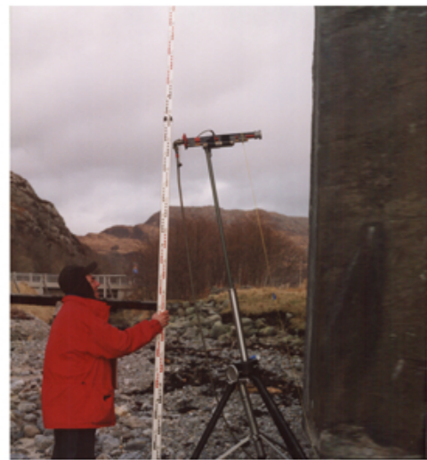
Loch-nan-Uamh Viaduct – Dr Stove scanning at north face centre pier © R. Paxton
