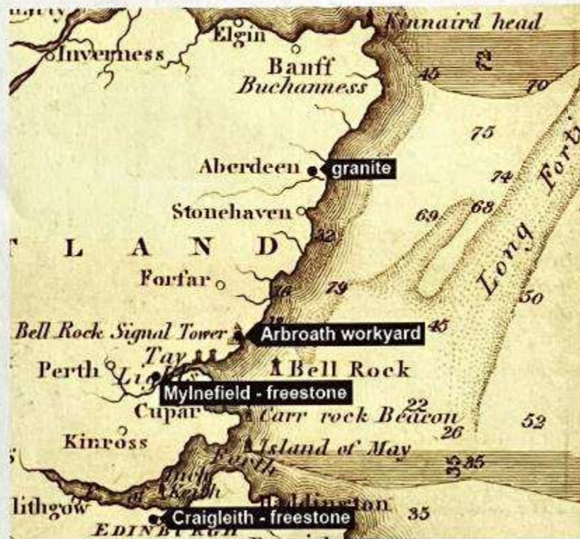
Fig. 2 Part of chart (1, pl. III) showing the lighthouse and stone sources Each of its 90 courses was prepared at Arbroath. In its mortars, Italian pozzolano, Aberthaw lime and Roman Cement from Kent were used
