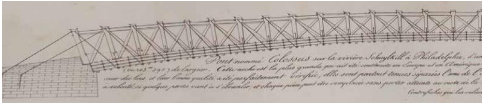
Fig 8 - Wernwag's magnificent timber/iron rod 'Colossus' arch of 340ft span at Philadelphia 1812 (destroyed by fire in 1838)
