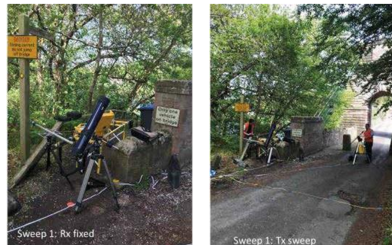
Fig. 3 [L] Location of Rx receiver mounted onto the Newtonian reflector telescope which is pointed directly at the 1903 downstream anchor plate at right angles to the plate. [R] Location of Tx bistatic ADR Sensor mounted on an astronomical motorized base tripod sweeping the 1903 plate from a depression angle (DA) of -51 to -42 degrees pointing from CH2.75 to CH3.0m along sweep line continuing to a DA of -16 degrees at chainage 4.75m
