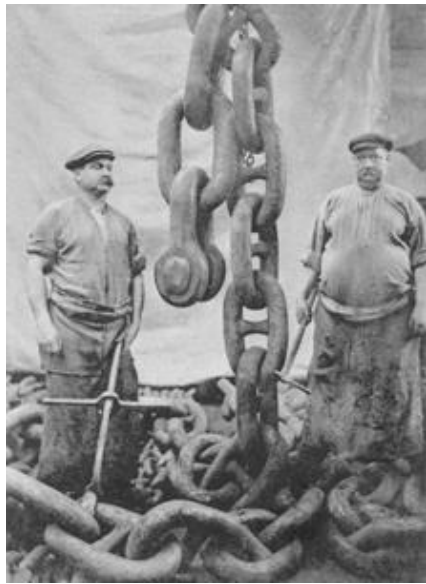
Record Ship's Cable in 1905 3¾ inch cable manufactured by Brown, Lennox & Co., Pontypridd, for the Quadruple Screw Turbine Express Steamer, built by Swan Hunter, and Wigham Richardson, Limited for the Cunard Company, Limited
