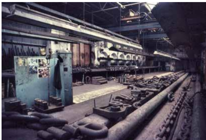
The Newbridge testing house, showing two hydraulic machines with the oldest (1868) machine on the left. Tested chain cable would be lowered through the floor into canal barges in the canal pond below. Photograph taken in the 1980s when specialist chain work including shackles etc. was still demanding the skills of Newbridge smiths. (SKJ photograph)
