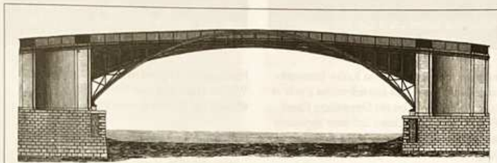
Fig. 4. Buildwas Bridge (1795) featured an experimental Schaffhausen suspension rib on each side and, at 40 m, was briefly the world's longest cast-iron span
