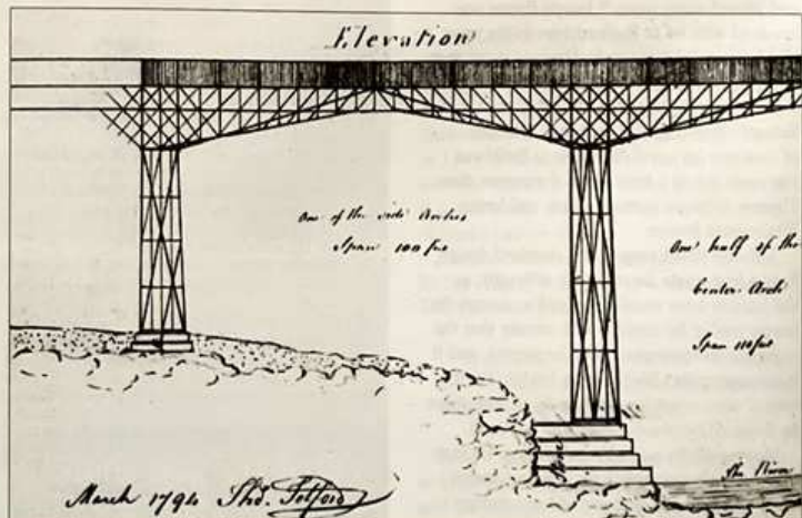
Fig. 1. Telford's preliminary 1794 cast-iron design for Pontcysyllte Aqueduct was based on timber truss design principles and had a main span of 33.5 m (Science Museum Library, London, No. 110, 592/61)
