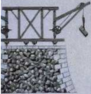
Transverse Section of the Pier in progress Showing the position of the crane and the manner of raising all the Materials & the Ballast.
