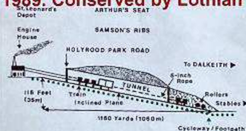
EDINBURGH AND DALKEITH RAILWAY Inclined Plane (1831) — Vertical Profile
