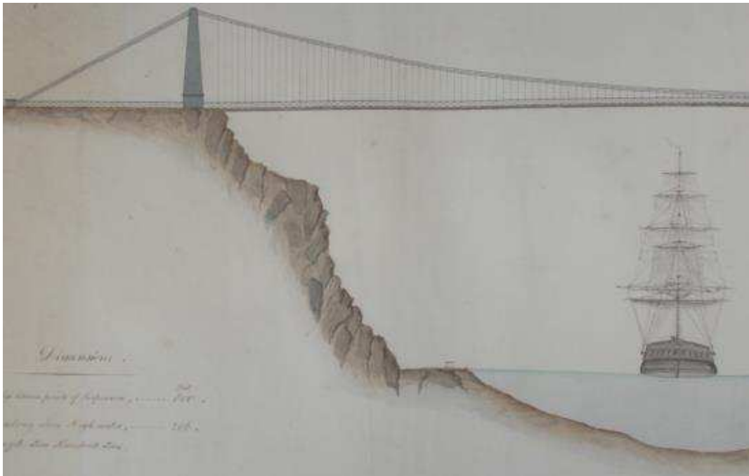
Drewry's drawing of Capt. Brown's Clifton Bridge Proposal 1829 [runner-up to Brunel's in Competition]
