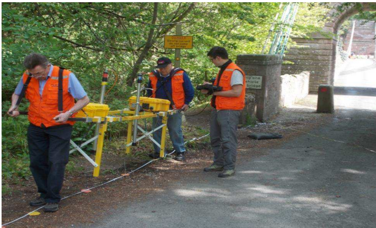
Survey crew led by Dr. Stove engaged on WARR scanning on line of bridge chains 17 May 2018 Note: Adrok designed transmitter and receiver on frame. High quality data was obtained which is being analysed and a report with findings is in preparation [see next Newsletter for results]
